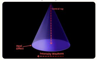
Point source tubes produce a non-symmetrical photon distribution, resulting in uneven intensity.
